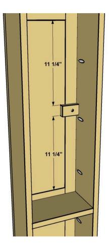
Note: Center Door Stop on opening. Glue and screw in place.
